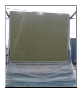
Water Penetration per ASTM E331
